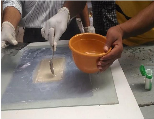
Fig hand layup process
