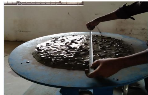
Fig-3 Slump flow test
