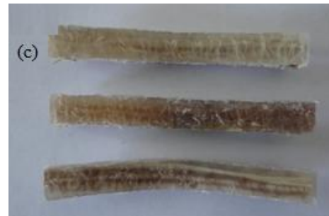
Fig. 13 Composite specimens after flexural strength test
