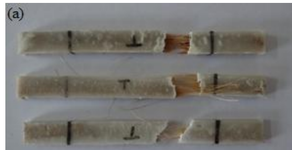
Fig. 9 Composite specimens after tensile test
