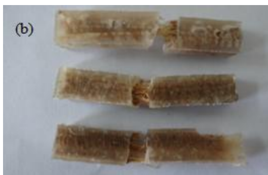
Fig 11 composite specimens after impact test
