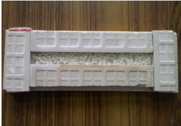
Fig.2 Mould for microwave curing
