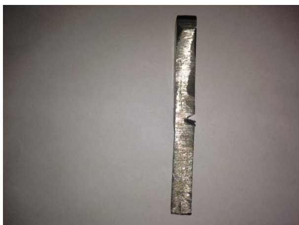
Fig.6: ASME standard sample with notch for Izod testing
