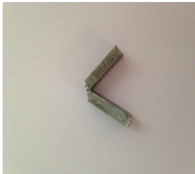
Fig.7: Sample after the Izod testing
