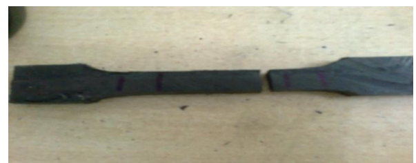
Fig. 4. Tensile test specimen after failure
