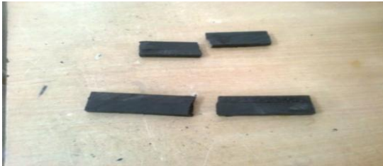
Fig. 6. Flexural test specimen after failure
