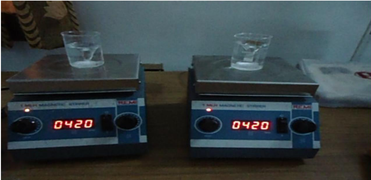
Fig.3: Stirring of the two mixtures ( \text{Zn}(\text{NO}_3)_2 and precursor KOH)
