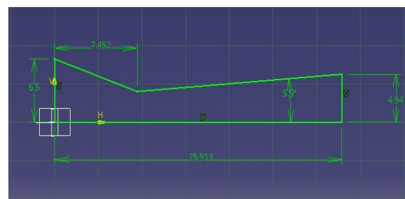
Fig-1: Sectional view of the nozzle at 11° angle of divergence
