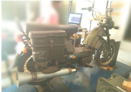
Fig.4 Chassis Dynamometer with CD Nozzle type exhaust
