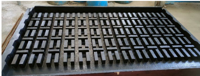
Fig 3.5 Prime coat and Colour coating to mould
