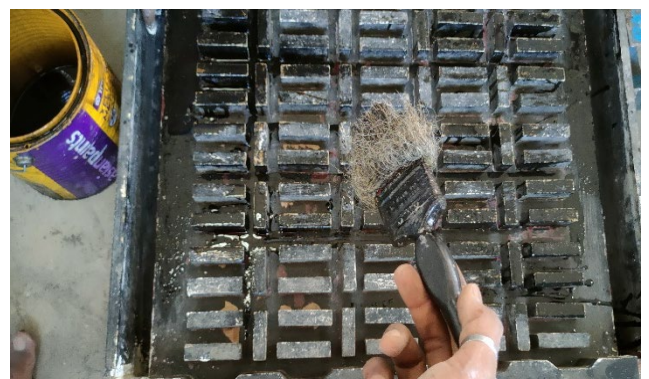
Fig 3.8 Oiling to mould
