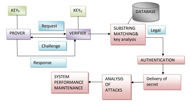
Fig 1: Block diagram for prover authentication and message transfer
