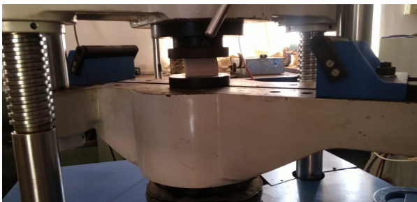
Compression test of WPC
