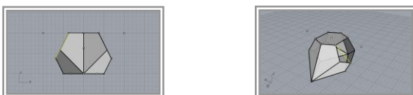
Fig. 15. Second cut. Just draw a line, get to a side viewport and trim the solid
