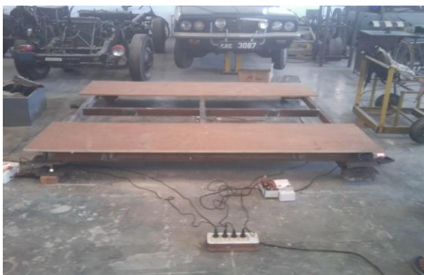
Fig. 4. Experimental setup of COG measuring using 4 load transducer method
