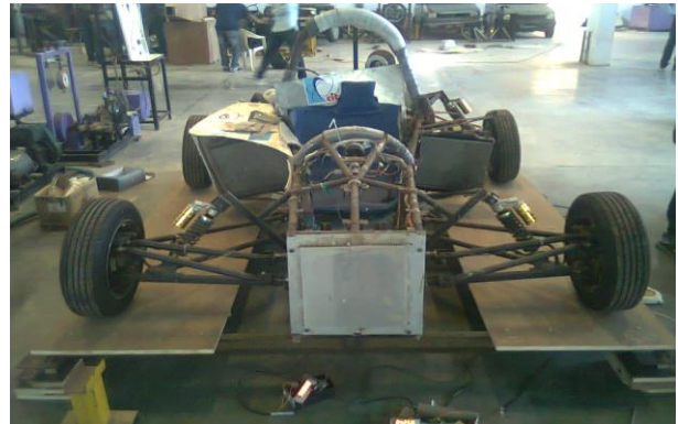
Fig. 5. Measurement of C.O.G. SUPRA SAE CAR
