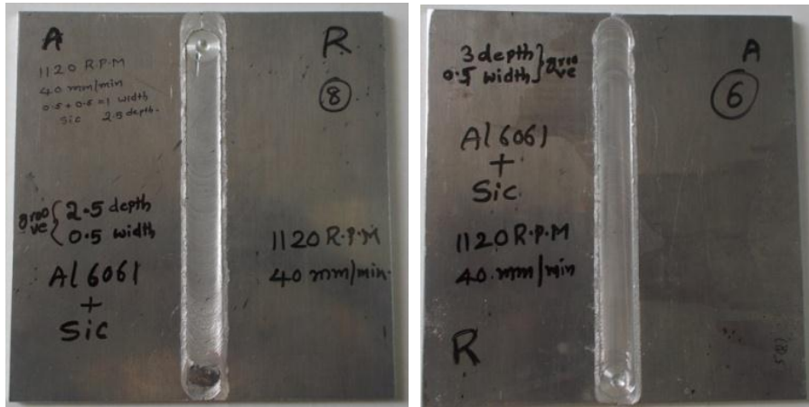
Fig.3: FSW Joint With 10% Sic By Volume Fig.4: FSW Joint With 15% Sic By Volume
