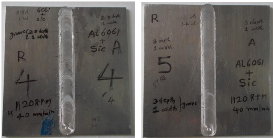
Fig.5: FSW Joint With 10% Sic By Volume
