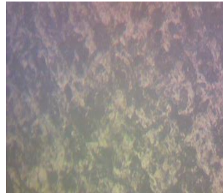
Figure 4. Microstructure of Al7005 with 3% S glass and 6% fly ash
