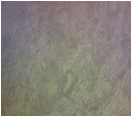
Fig 2. Microstructure of Al7005 with 1% S glass and 6% flyash
