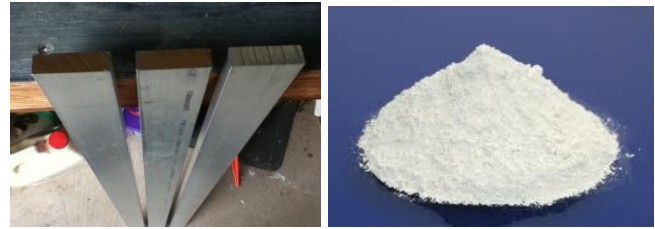
Fig. 1. Aluminum 6061 bars and ZrO 2 in powder form used for the preparation of composites.
