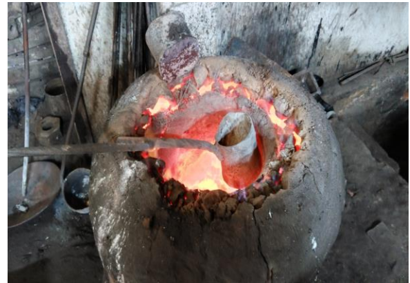
Fig. 2. Furnace used for melting the Al6061 rods.
