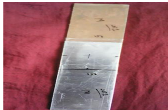
Fig. 2. Assembly of lap configuration of the joint
