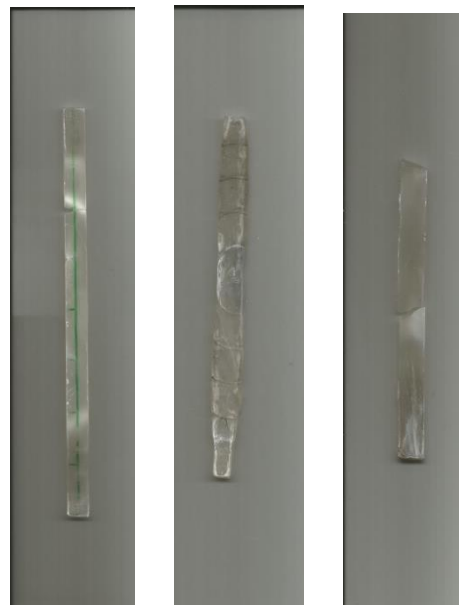
Tensile Specimen Compression Specimen Bending Specimen
