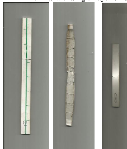
Tensile Specimen Compression Specimen Bending Specimen
