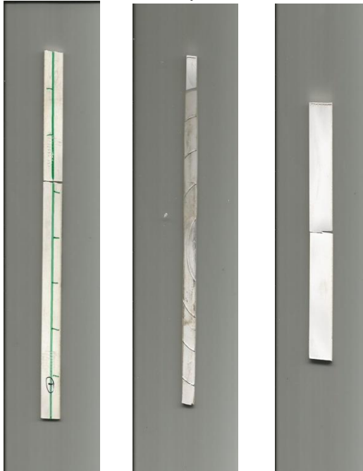
Tensile Specimen Compression Specimen Bending Specimen
