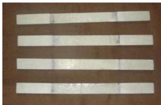
Figure 1 : Specimen prepared & cut for tensile test
