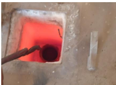
Fig. 4.1 Preheating of Particulate Reinforcements
