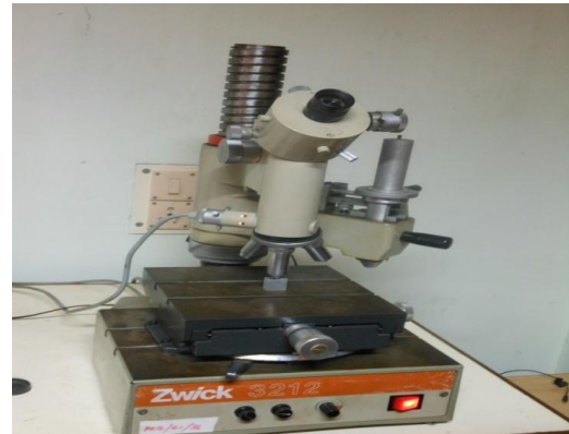
Fig. 5.9 Pictorial view of Vickers's Microhardness Tester used
