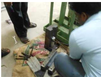
Fig. 4.5 Removal of cast samples from die
