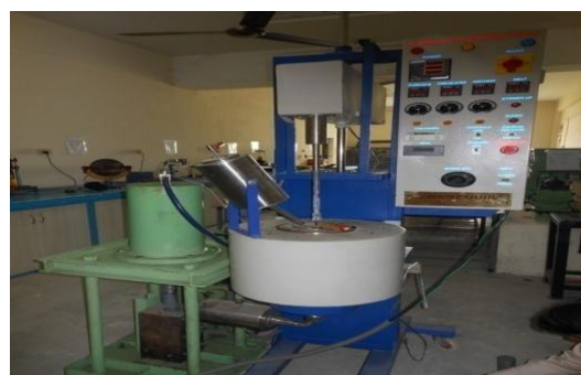
Fig. 4.3 Squeeze casting machine used
