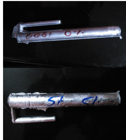
Fig.1. shows cast die, Al6061 and Al6061 + 5wt% AIB2
