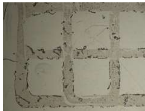
Fig. 2. Channel fabricated channel by using PDMS and SU8
