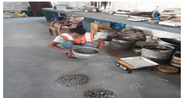
Fig No: 3 Trial & Error method for fixing blending proportions
