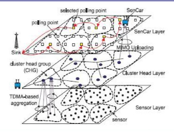
In The above figure shows the Three sensor layer frameworks such as Sensor layer, Cluster head layer, mobile collector (Sencar)layer. The sensor layer is the bottom layer of the sensor network.in which the sensor nodes are deployed in this layer. The second layer is the cluster head layer in this layer the sensor nodes creates the cluster head on the basis of energy node. In the sencar layer the created head nodes applying the load between two nodes it maintains the load.
