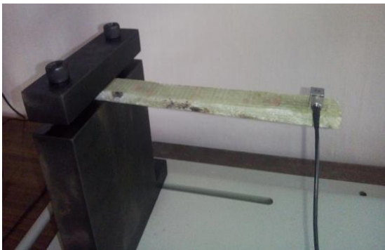
Fig.2 Cantilever composite beam test set up
