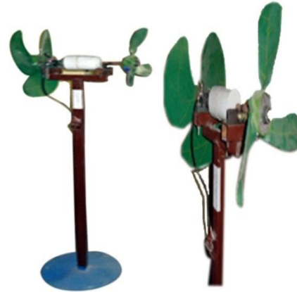
Figure 4. 0.373 kW (0.50 H.P) Prototype test model of PMSLCRWPG
