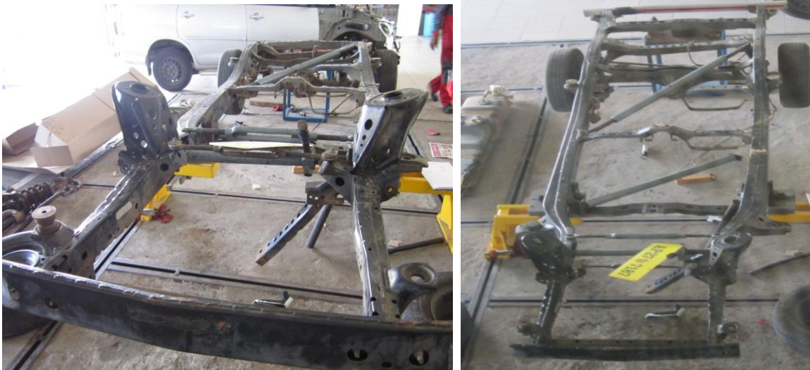
Fig(c&d).shows the real model of innova car chassis frame
