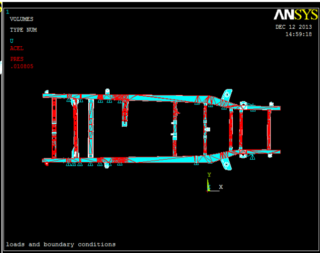
Fig(2). Loads and boundary condition
