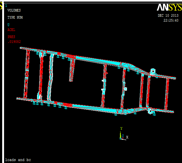
Fig(9).loads and boundary conditions
