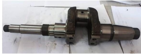
Fig.1. Single Cylinder Crankshaft to be Modeled using Creo Parametric
