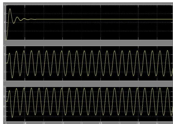
Figure 12 – Buck converter & inverter (across load) output
