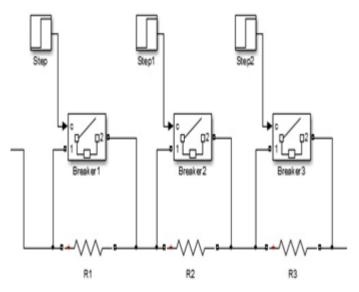
Each breaker are connected in parallel with the specific resistance, these are arranged in series with the armature winding. Initially for breaker 1 are in open '0' position which are step with particular time interval to '1' position and resistance R1 are by-passed with the short circuit. R1 is cut down from the external resistance. Similarly R2 and R3 by breaker 2 & breaker 3 are also cut down with particular time interval with each other. The whole resistances are cut down in three steps.
