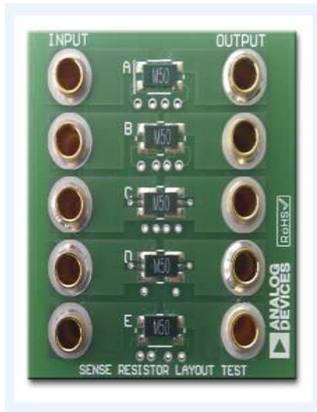
Fig. 4. Sense resistor layout test PCB.
