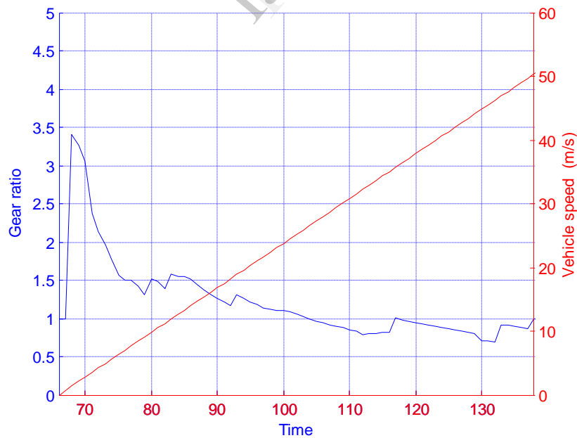
Figure 11. Gear ratio selection for maximum motor efficiency for a constant acceleration of 0.7 \text{ m/s}^2
