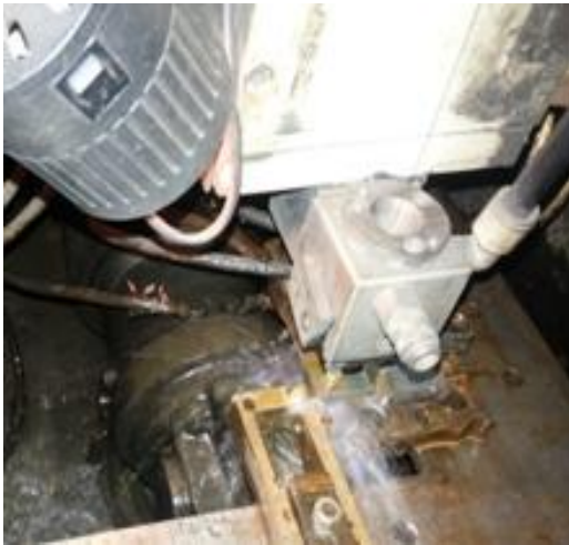
Fig .II Working zone of wire EDM
