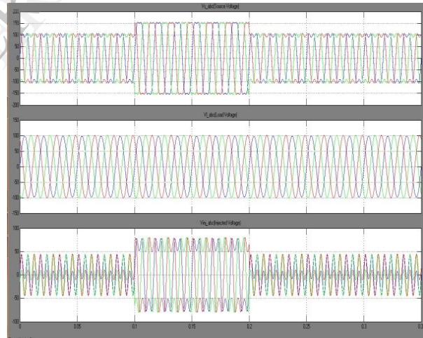
Fig.13. input distorted and swell Voltage, Compensated Load Voltage and Injected Voltage with Swell condition
