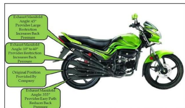
Fig. 2. Effect of change of exhaust slant on back pressure
