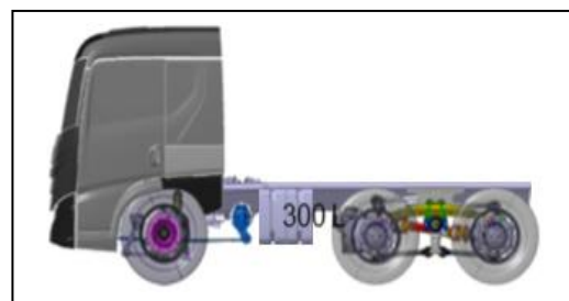
6x4 Tractor from 4x2 Haulage; Addition of rear axle, change in rear suspension, Fuel tank capacity change, cab type and frame
