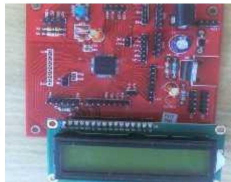
Figure 4.1: Renesas RL78 microcontroller with LCD display
