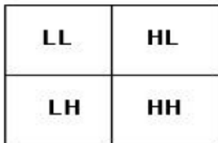
Fig. 1. Sub-band decomposition of Image
