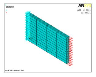
Interlaminar stresses ,and are responsible for delamination growth. For the above FE model the distributions of interlaminar stresses across the width of the plate.
