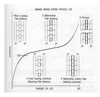
A schematics picture of damage development in fibrous composites.
