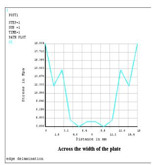
Variation of interlaminar shear stress ( $\sigma zz$ ) across width of the plate without cups for the ratio Gxy/Gyz =5
