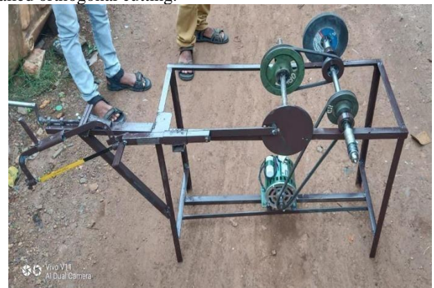
Fig 2: Cutting mechanism (Hacksawblades)
