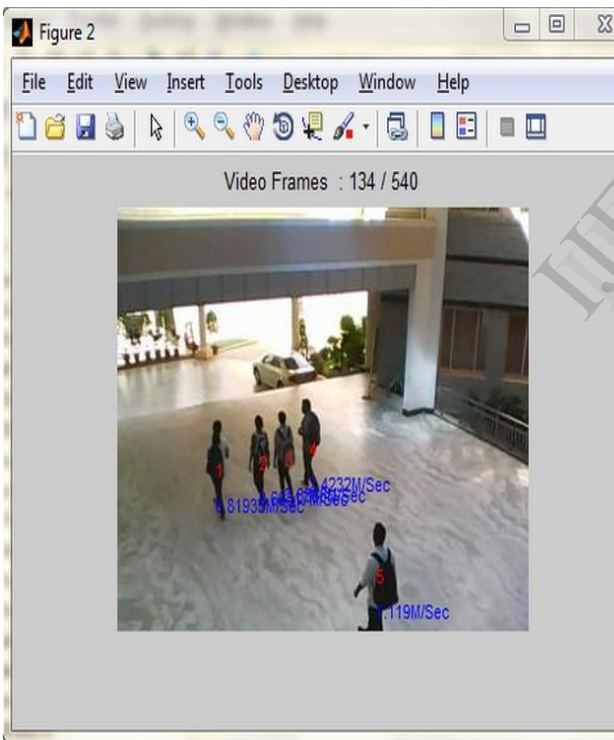
Figure 2a shows the output after frame difference, which contains five people moving with respective velocities.
