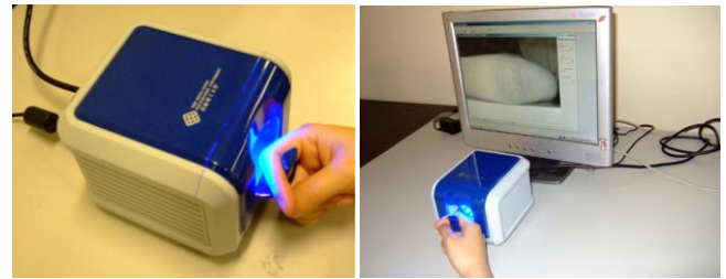
Fig. 2. (a) The outlook of the developed FKP image acquisition device and (b) the device is being used to collect FKP samples.
