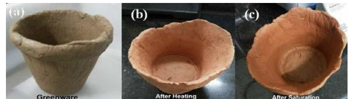
Fig. 11. Images of ceramic pot (a) Green ware (b) After calcinations at 800 °C for 5 h (c) After saturation
