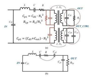
By using the electrical equivalent circuit the voltage gain characteristics of tunable piezoelectric transformer will be derived. The voltage gain characteristics of tunable piezoelectric transformer will depend on load operating frequency and input voltage.
