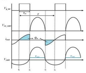
There will be some of the key waveforms in the control terminal the effective value of the capacitor will be determined by the charging and discharging time interval of an external capacitor. By assuming an sinusoidal nature of current the effective value of capacitance can be derived. By using an equation the duty cycle of the control MOSFET can be varied.
