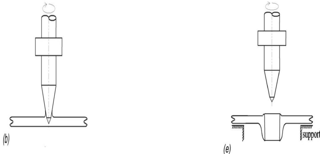
Figure 2, shows the different stages of the friction drilling process
