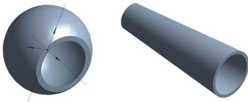
**Fig. 6 Geometric Model of spherical and conical receiver**
