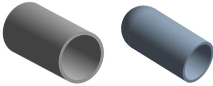
**Fig. 5 Geometric Model of cylindrical dome receiver**
