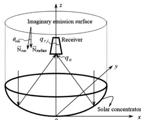
Fig. 1 Schematic diagram of the dish solar concentrator/cavity receiver system
