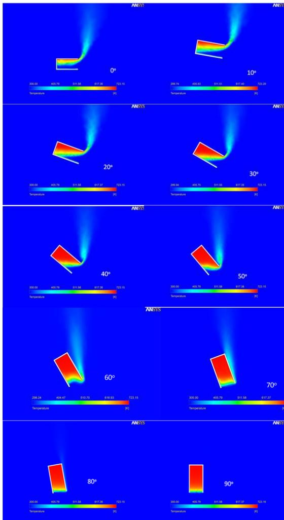
Fig. 9 Cylindrical receiver Temperature contours at inclination  $0-90^{\circ}$
