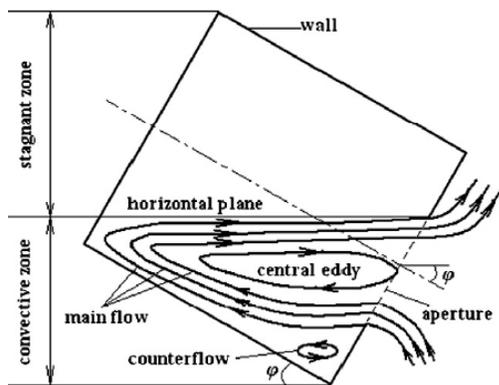
**Fig. 3 Stream Lines in Upward Facing Tilted Cavity Receiver**
