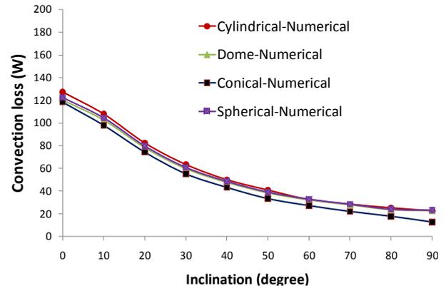
**Fig. 18 Convection Heat loss comparison**
