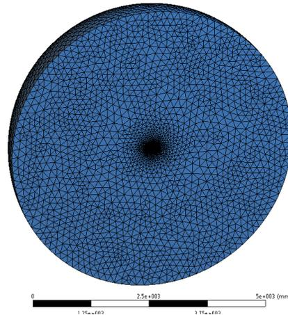
**Fig. 7 CFD Domain of dome receiver**
