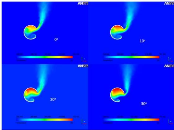
**Fig. 16 Spherical receiver Temperature contours at inclination 0-30°**
