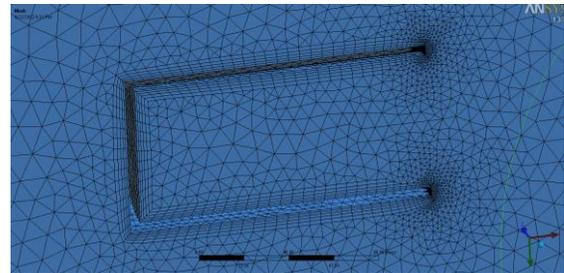
**Fig. 8 Boundary layer Mesh close to cylindrical receiver wall**
