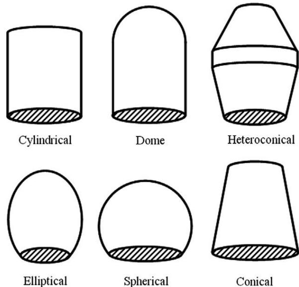
**Fig. 4 Six classical cavity geometries**
