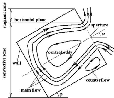
**Fig. 2 Stream Lines in Downward Facing Tilted Cavity Receiver**
