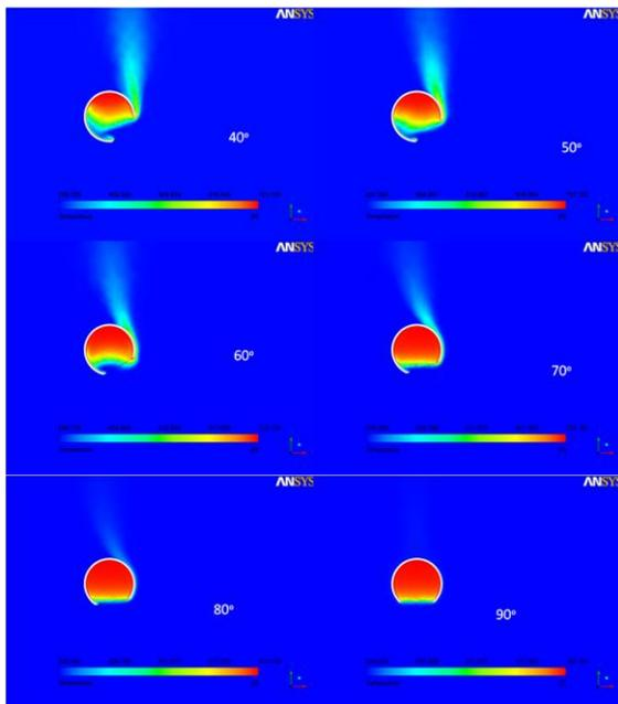
**Fig. 17 Spherical receiver Temperature contours at inclination 40-90°**
