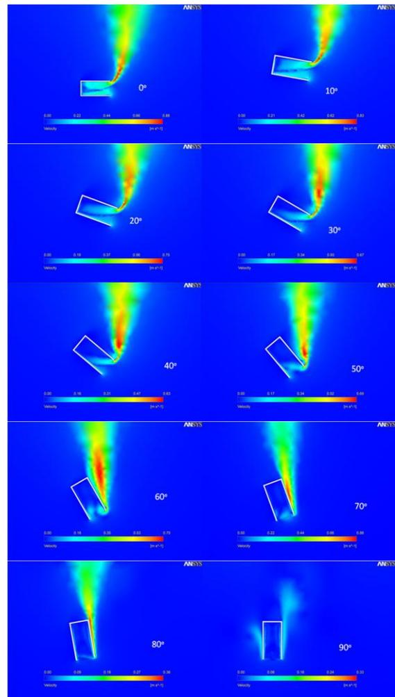
Fig. 11 Cylindrical receiver Velocity contours at inclination  $0-90^{\circ}$
