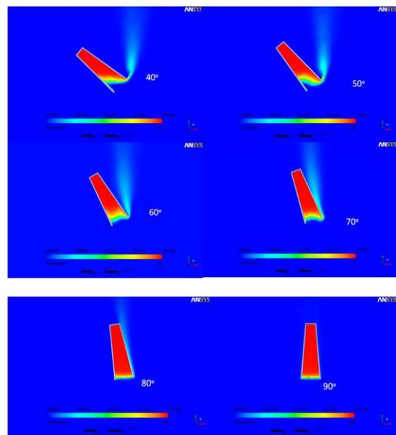
**Fig. 15 Conical receiver Temperature contours at inclination 40-90°**
