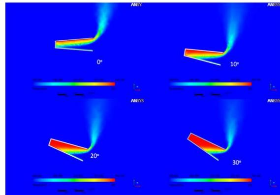
**Fig. 14 Conical receiver Temperature contours at inclination 0-30°**
