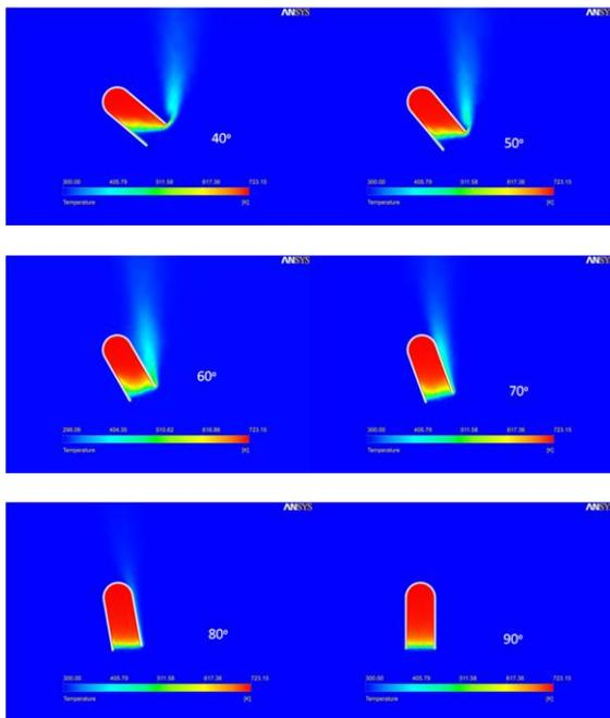
**Fig. 13 Dome receiver Temperature contours at inclination 40-90°**
