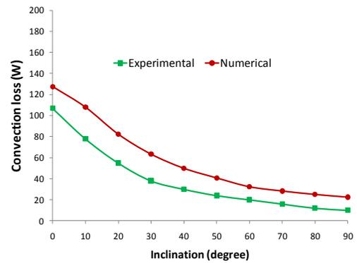
Fig. 10 Comparison of Experimental and Numerical values for cylindrical receivers
