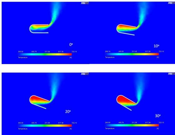
**Fig. 12 Dome receiver Temperature contours at inclination 0-30°**
