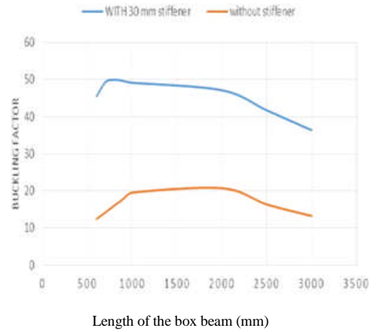
Fig 7 Comparison of buckling factor of the box beam with and without the stiffeners
