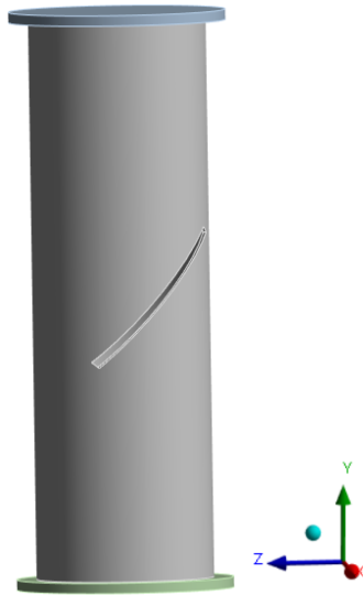
Fig. 2. Column with oblique notch modeled in ANSYS.
