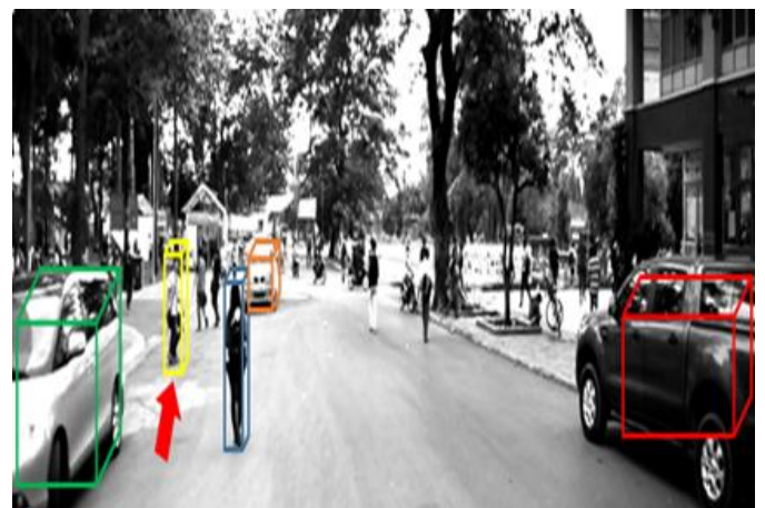
Figure 7. Object detection, tracking and recognition. a) and b) are results of the campus data.
