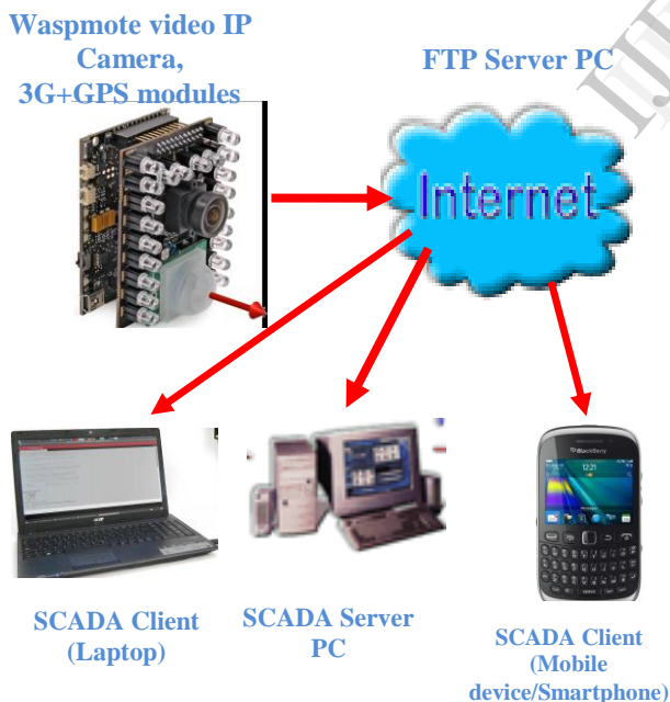
Fig.13. The functional block diagram showing interactions amongst FTP, MySQL and Apache Web Servers with SCADA users
