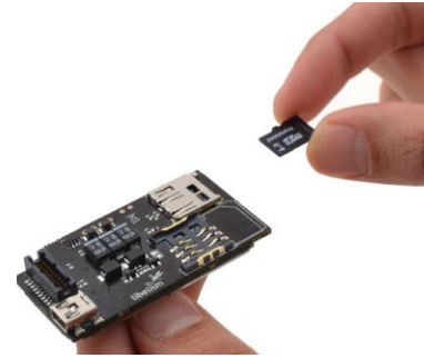
Fig. 10. The Transcend microSD™ 2G card used in the project being inserted into the Waspnote 3G sub-module
