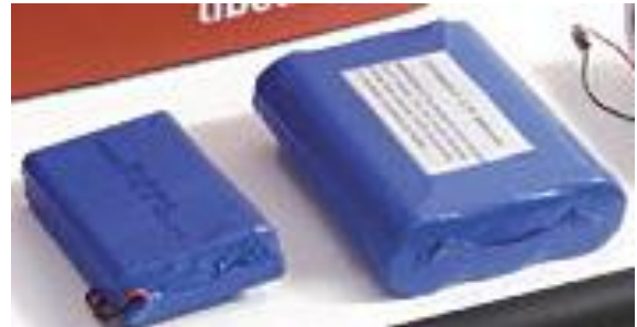
Fig.14. The 6600mAh rechargeable battery used to power the entire hardware sub-system
