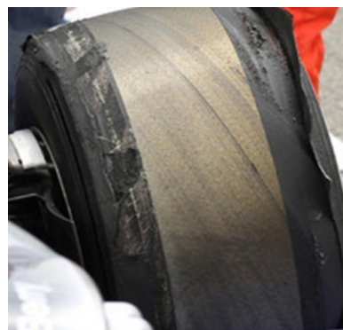
Fig 1.6 – Removal of tire thread
