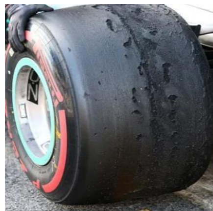
Fig 1.3 – Tire wear due to camber
