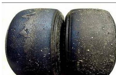
Fig 1.7 – tire wear due to pressure
